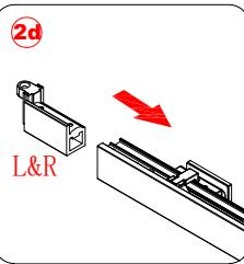
If it is installed on the left, use the left connector, and if it is installed on the right, use the right connector
